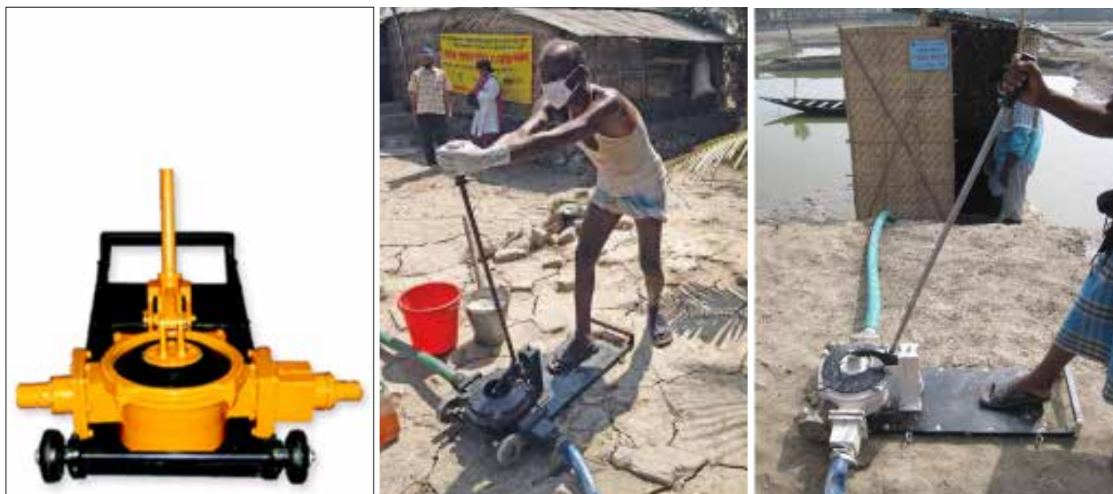
Figure 25: Manually Operated Diphragm Pump used in Bangladesh
