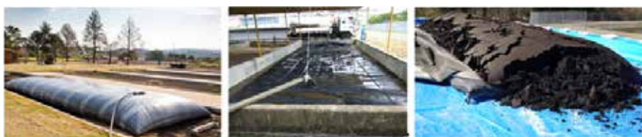
Figure 45: Geobags and its Application for Solid -Liquid Separation
